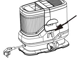
3. Detache the water tank by lift it upwards.
