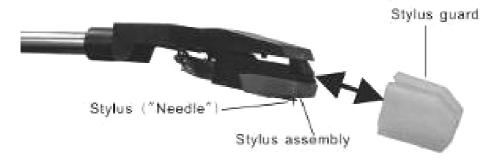
Remove the stylus guard gently from the needle and put back the security latch.
