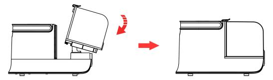
Put the dust container along the direction of the arrow in the figures.
