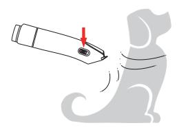
Slide the power switch to turn the clipper on and off. The clipper only works when the vacuum is switched on.
