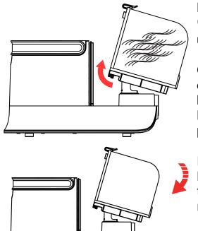
Press the dust container release button (a) and detach the bin from the vacuum unit.
