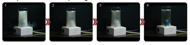
Blow smoke into the glass.  $\rightarrow$  turn on the ionizer.  $\rightarrow$  the smoke starts to vanish.  $\rightarrow$  the smoke is completely removed in a few seconds.
