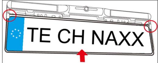
**3.** Insert the top cover strip's clips into the relative holes of the license plate holder then press tight.
