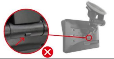
Choose a right place on the windshield and mount the suction cup mount on the windshield. With the suction lever in the released position, press the suction cup against the windshield. Press the suction ever toward the suction cup to lock the mount adjust the To angle monitor, loosen the collar on the ball joint, retighten in the desired position.
