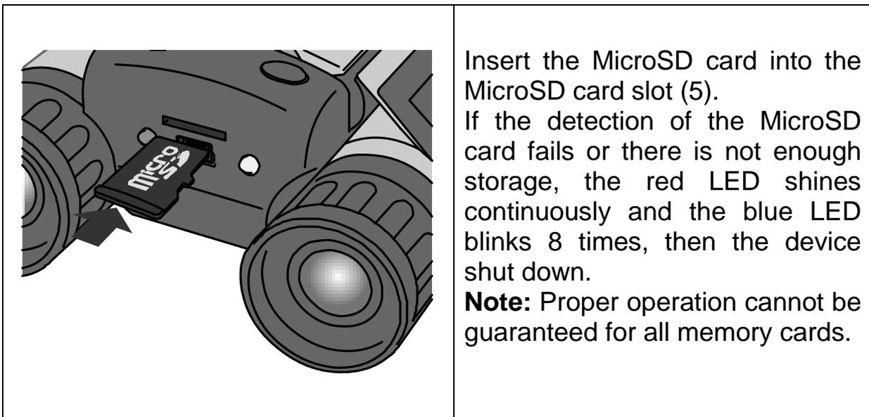
Insert the MicroSD card into the MicroSD card slot (5).
