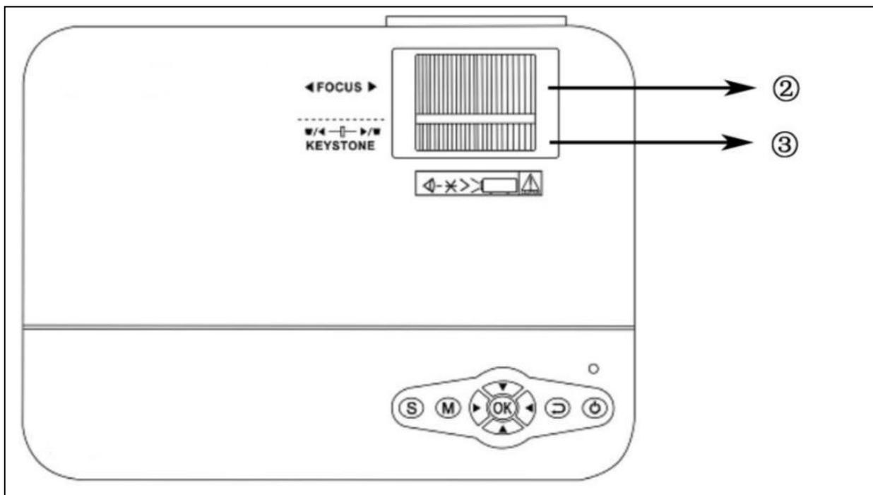
The device provides optical keystone function, so you could turn the keystone to adjust the image. The device does not have horizontal keystone correction function.
