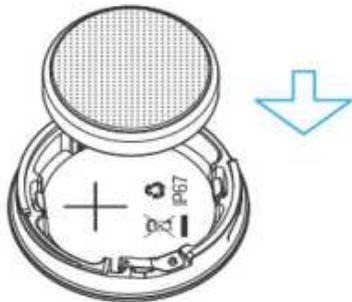
**02** Align the battery compartment at the front cover as below.
