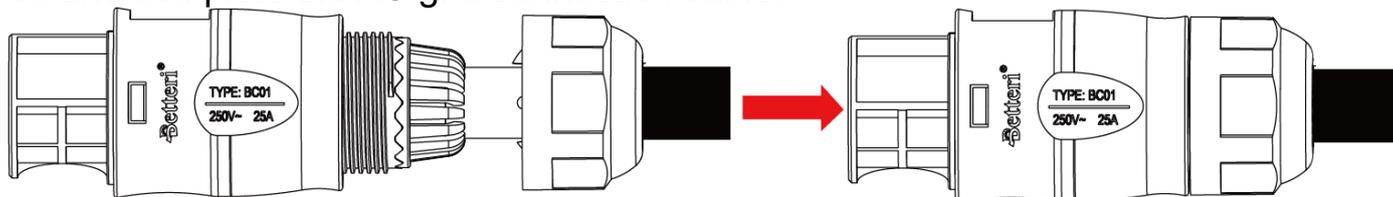
Connect the AC grid connection cable to the AC male connector of the first micro inverter to complete the circuit.
