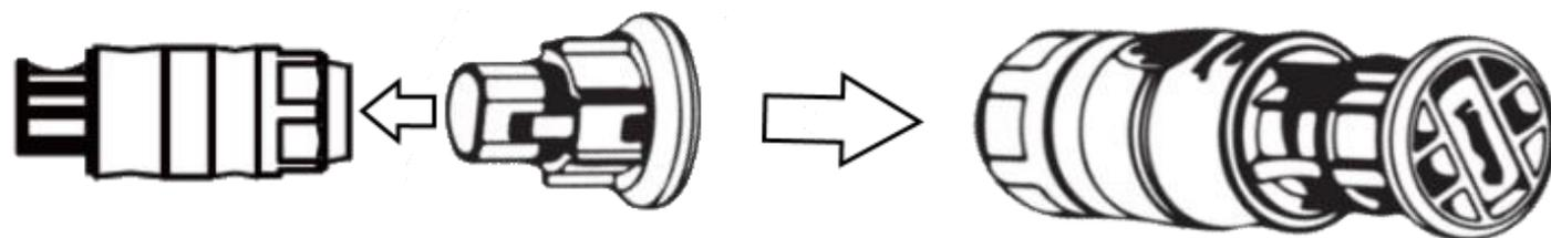
**Connect AC grid connection cable**
