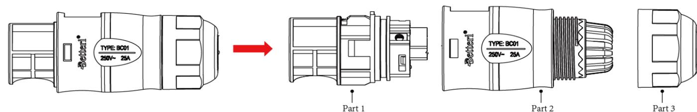
2. Insert the AC cable from Part 3 to Part 2, and complete the wiring for the L, N and Ground (PE) inside Part 1 AC port accordingly:
