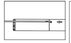
Place the small barbed hook of the attachment into the opening provided at the end of the gooseneck just below the camera head.
