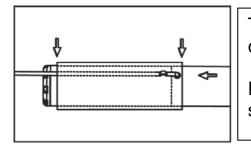
Then slide the attachment fixture carefully and completely over the camera head.
