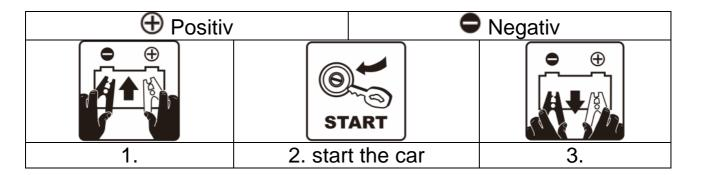
**First (1.)** → put the red clamp to the positive pole (+) of car battery (maximum contact area), then put the black clamp to the negative pole (–) of car battery (maximum contact area).
