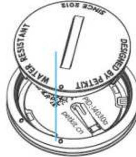
**03** Screw the battery cover with the opener clockwise to the end.
