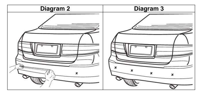
Rear Sensors A, B, C, D should be mounted from left to right with A being the leftist side and D being the rightist side.
