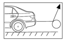
Spherical objects have a small and uneven surface area, due to the curvature of spherical object the signal reflected away, maybe.
