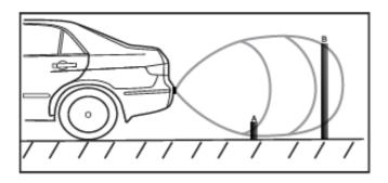
Obstacle A is of low high. Therefore during reversing, obstacle A will be detected initially, until obstacle A enters the sensor blind zone. Once obstacle A is in the blind zone, obstacle B will be detected. So you must be aware although obstacle A is no longer detected, it is still there!
