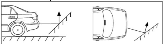
In case of small angle of incidence to the obstacle, such as Glass or other smooth plane, the obstacle may not be detected as the signals are reflected away.
