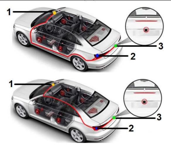
The 2.5mm plug needs to be plugged in the AV IN of the mirror. Camera plug and the red cable of the camera need to be directed to the back of the car. Connect the red cable with the positive pole of the reversing light.
