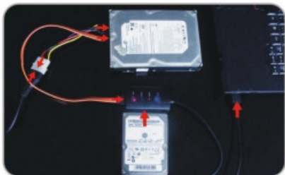
1.USB-Adapter to Multi-Function IDE/SATA(support 2.5" Hard disk) 2.Power Adapter
