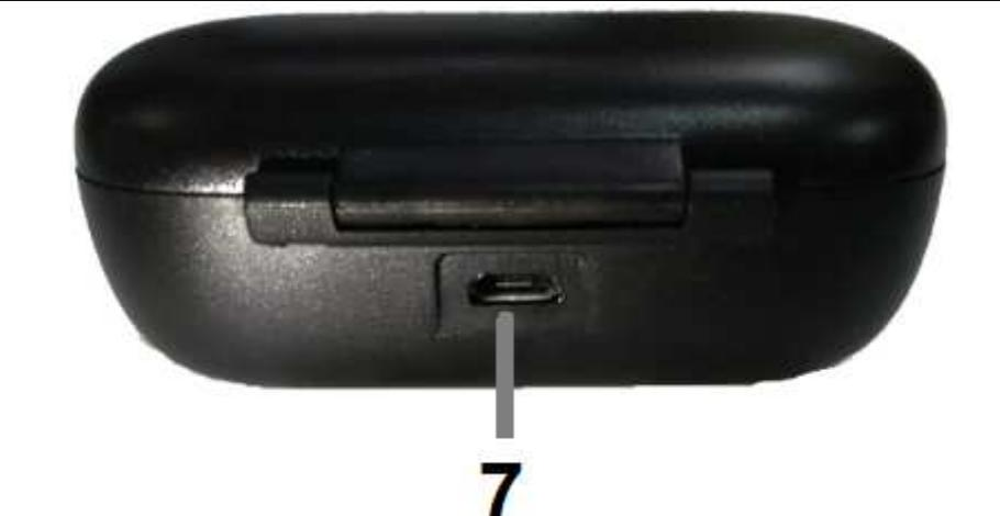
The image shows the back view of the closed black charging box. A small Micro USB connector is visible on the bottom edge, indicated by callout 7.
