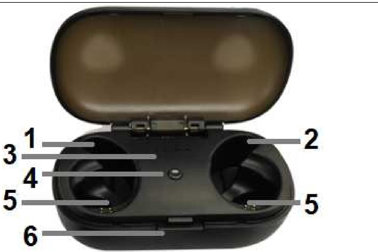
The image shows the front view of an open black charging box. The lid is flipped up. Inside, there are two earpiece compartments. Numbered callouts are as follows: 1 points to the left earpiece, 2 to the right earpiece, 3 to a small display on the left side, 4 to a small circular button in the center, 5 to the charging contacts in both compartments, and 6 to a small rectangular button at the bottom.
