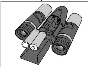
Remove the battery cover (8) on the back of the device. Insert two LR6) AA (1.5V)batteries observing the correct polarity indicated. Close the battery compartment with battery the cover.
