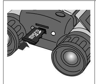
Insert the MicroSD card into the MicroSD card slot (5).
