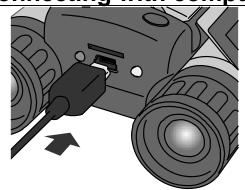
Please connect the Mini-USB cable with the device as shown in the left picture. Please connect the other end with the computer. If the device is connected to the computer, it enters the USB-Mode automatically. The red LED shines and the blue LED blinks.
